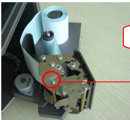
(5) Roll the release paper in the rewriter axis, and adjust the paper-fixing-block to fix the roll paper.
